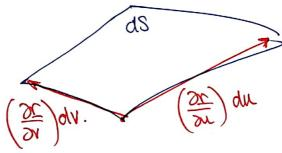
The result of  $dS = |C_u \times C_v|$  and follows by area of ponallellogram
